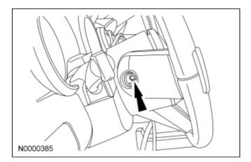
4. Disconnect the 2 driver air bag module electrical connectors and remove the driver air bag module.
